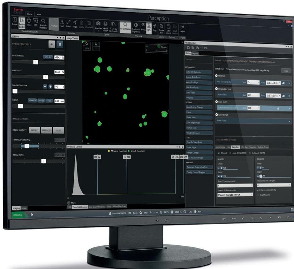
Perception Software uses recipes to create a standardized way of working. To help you get started, it includes several industry-specific workflows based on years of particle analysis experience. These workflows include three primary recipes:
