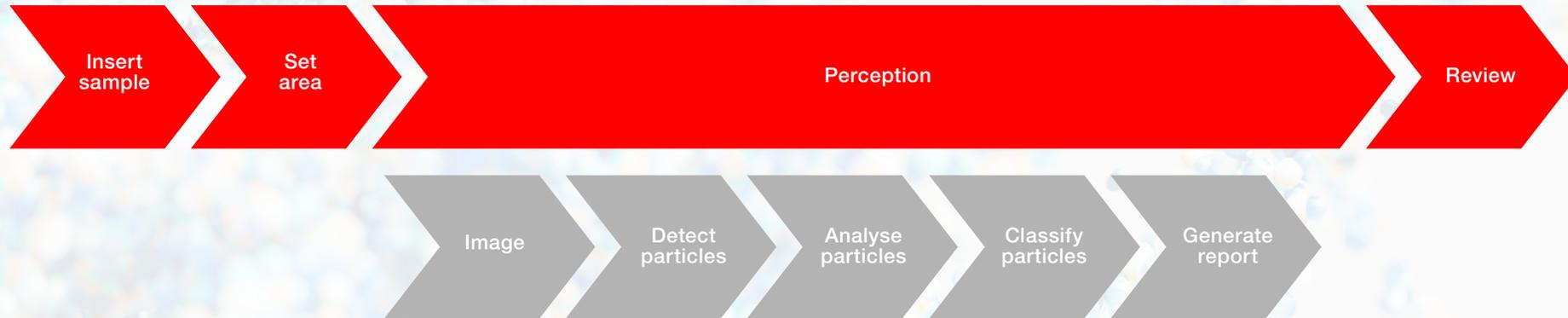
Perception Software automates many steps of the particle analysis workflow, reducing time spent on manual tasks.
