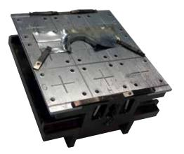
Figure 1: Picture of the aluminum sample mounted on the K-Alpha sample block
