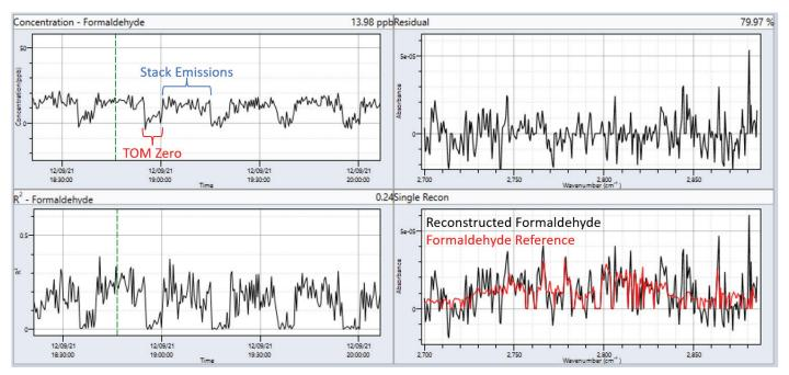
Figure 1: Formaldehyde measurements collected in the field from a natural-gas fired turbine engine.
